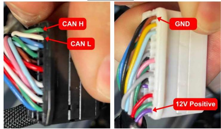
**Note:** The **grey & blue** and **white & brown** wires must be twisted together before they are joined to the original vehicles wiring harness.
