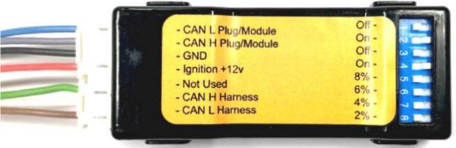
Identify the wires on the speedo corrector as per the picture.
