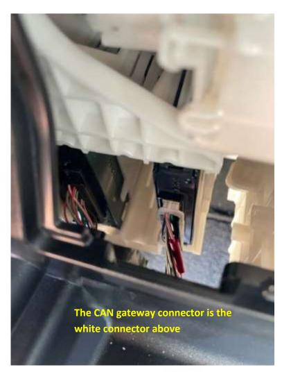
Unplug the white CAN gateway connector and feed it below the glovebox into the footwell.
