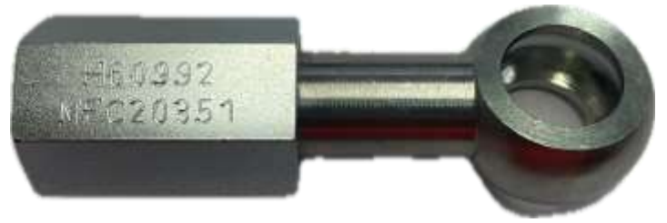
Image 3.4 Power steering sensor adaptor
