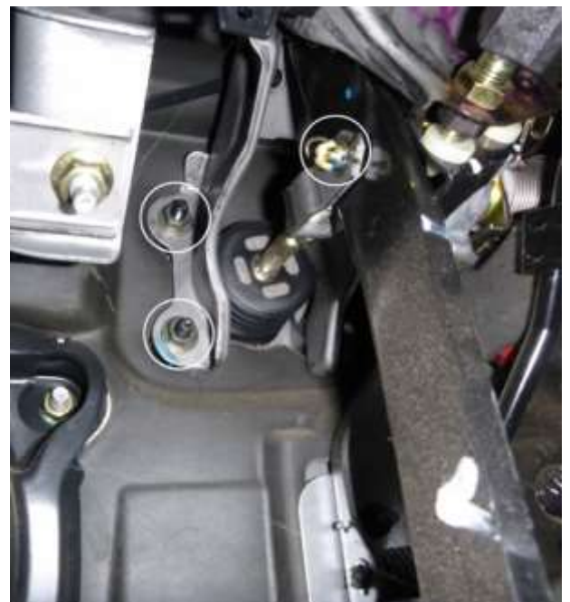
Image 1.3 Removal of the cotter pin and nuts.
