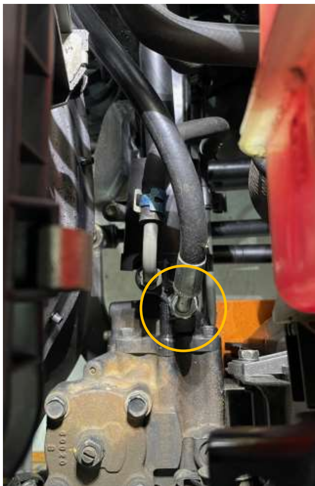
Image 3.2 Power steering box —45° hose fitting
