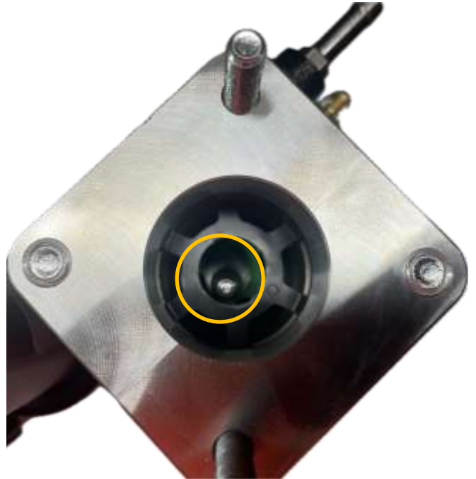
Image 2.1 Make sure the push rod is fitted in the hydro booster
