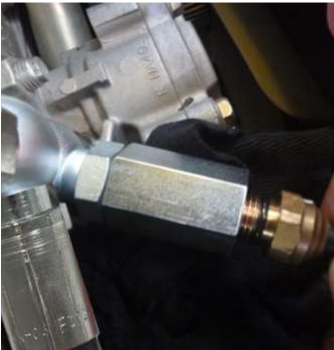
Image 3.8 Fit power steering pressure sensor
