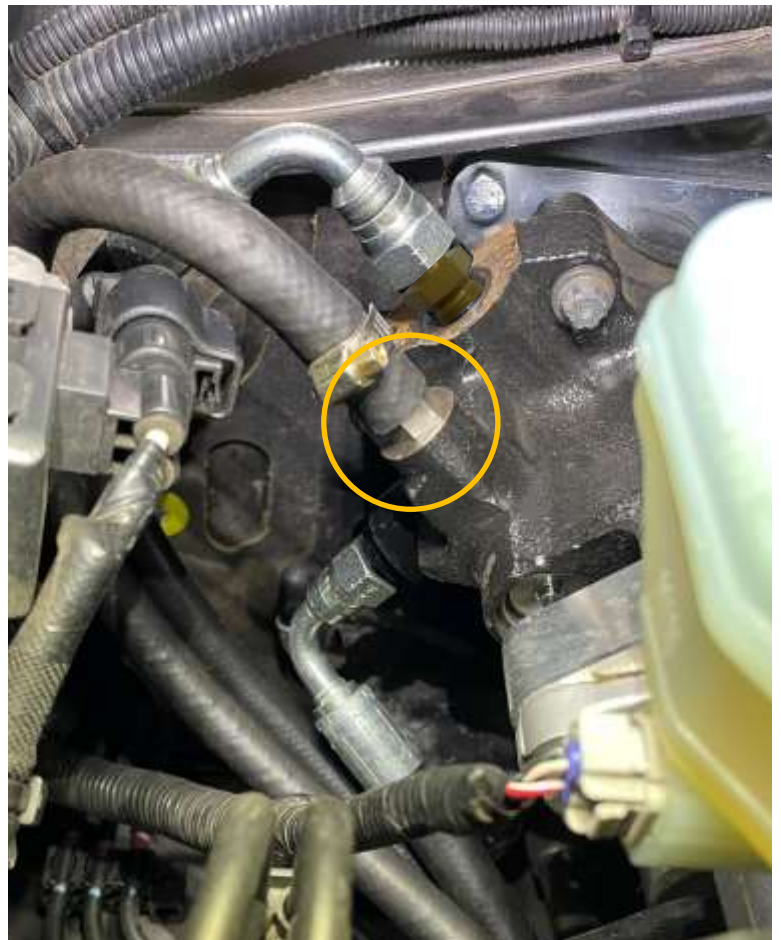
Image 4.0 Power steering box —45° hose fitting
