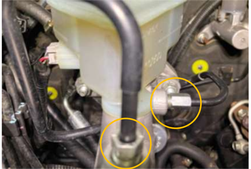
Image 1.1 Disconnect the solid brake lines
