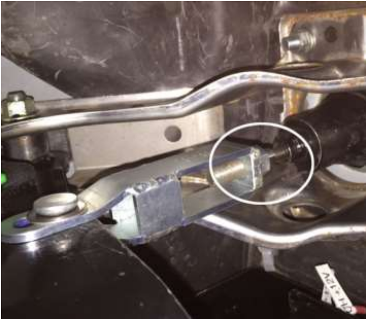
Image 2.4a Adjust the pedal saddle
