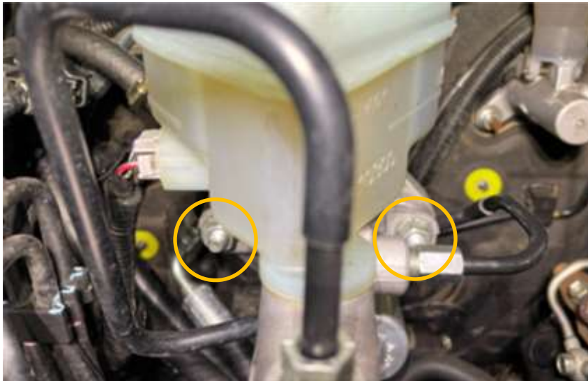
Image 1.2 Remove nuts holding master cylinder to booster
