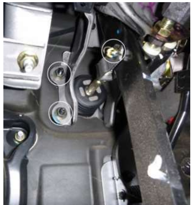
Image 1.3 Removal of the cotter pin and nuts.
