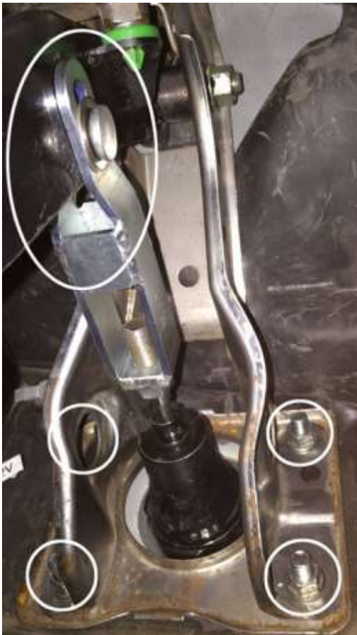
Image 2.2 Alignment of booster.
