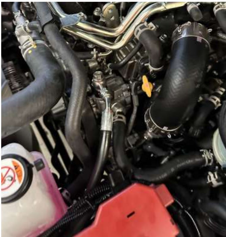
Image 3.8 Power steering pump fitted with new hose
