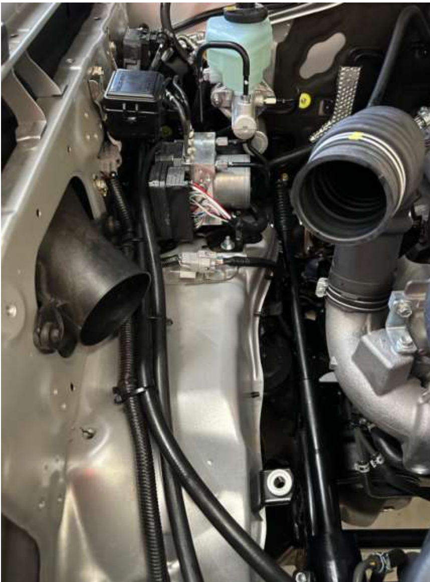
Image 3.4 Line routing behind ABS unit
