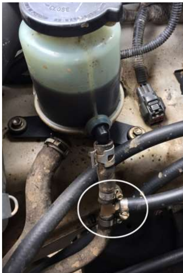
Image 4.1 Power reservoir tee
