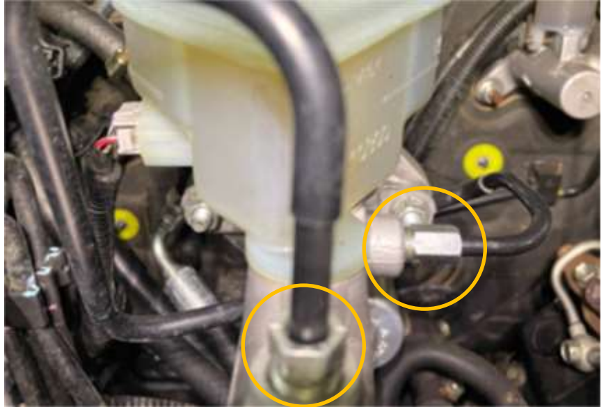
Image 1.1 Disconnect the solid brake lines
