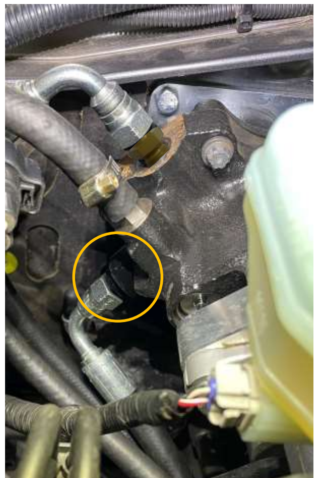
Image 3.5 Hydraulic booster—90° hose fitting
