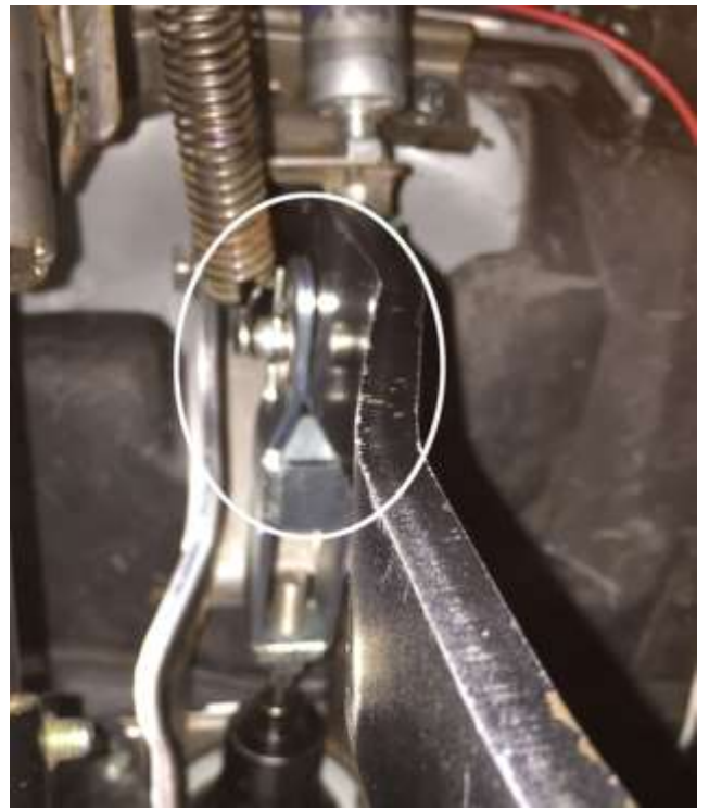
Image 2.3 Cotter pin install
