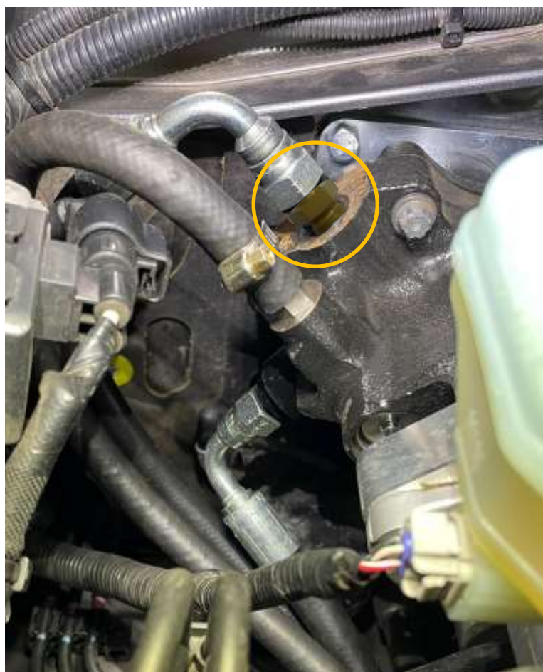
Image 3.3 Hydraulic booster—90° hose fitting
