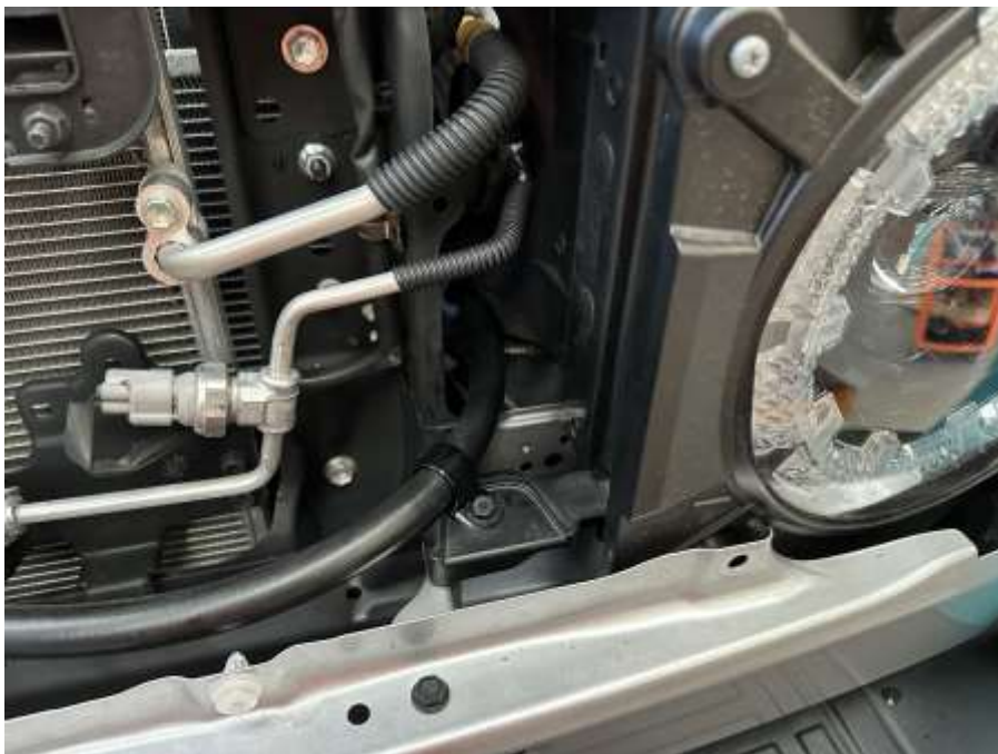
Image 3.6a,b,c Power steering line routing
