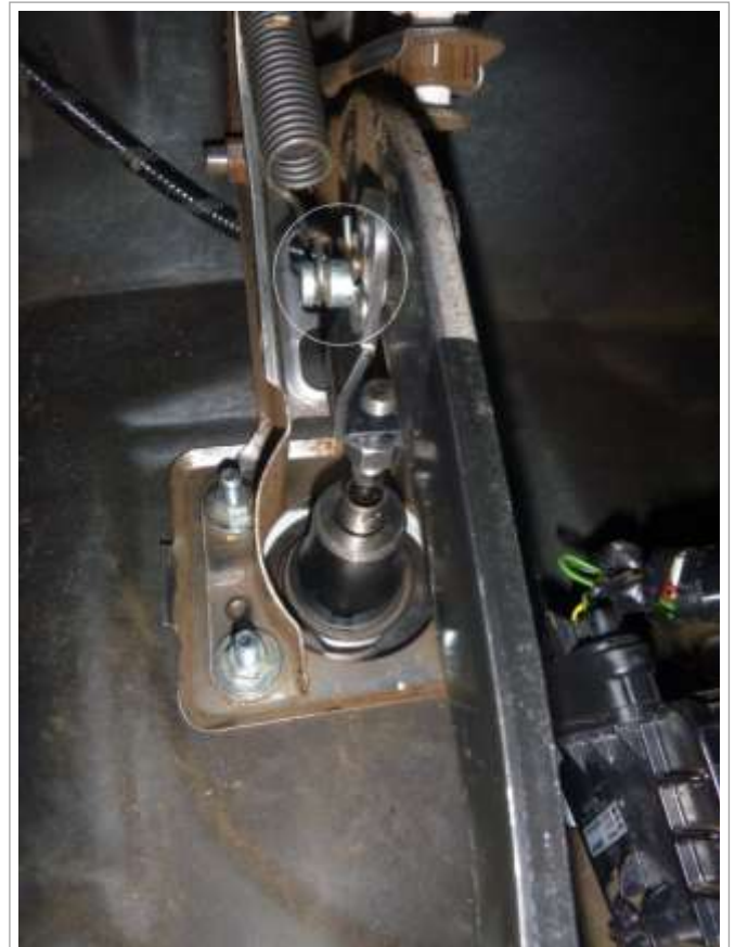
Image 3.2 Cotter pin install
