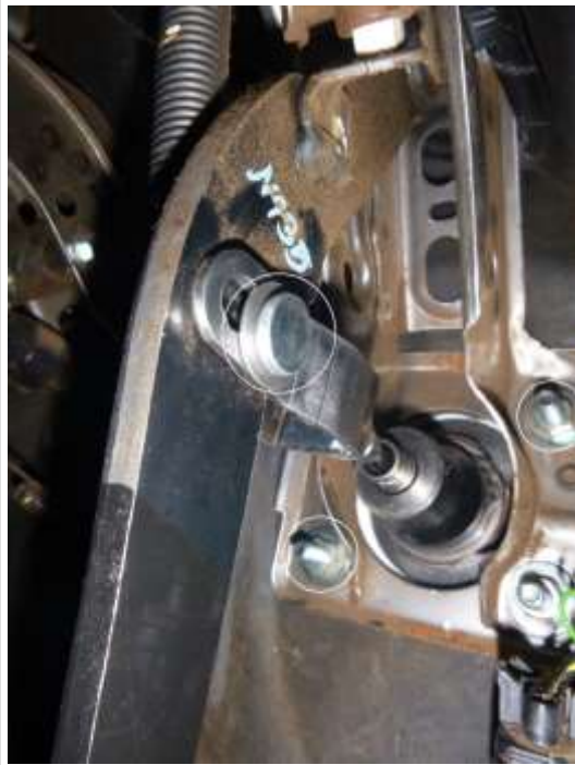
Image 3.1 Alignment of booster.
