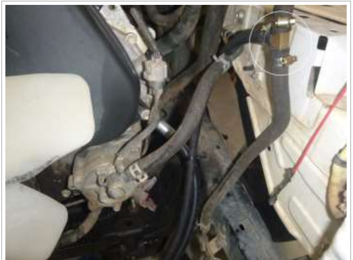
Image 4.6 Fitment to power steering reservoir bottle
