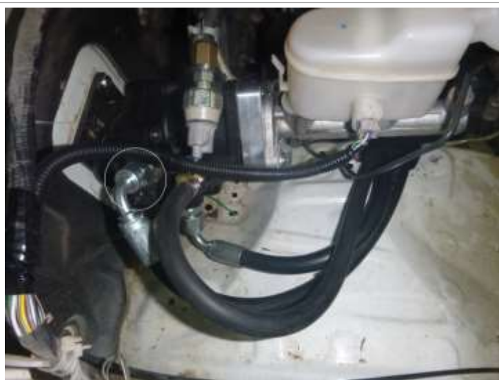
Image 4.2a Gold fitting on Booster (to steering rack)
