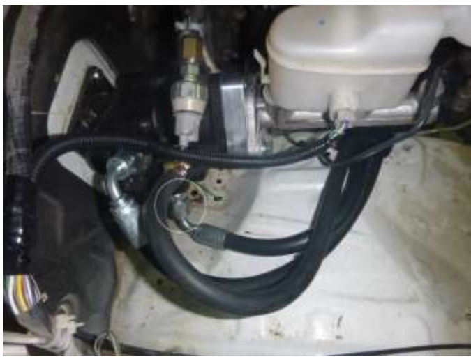
Image 4.3 Booster to power steering pump
