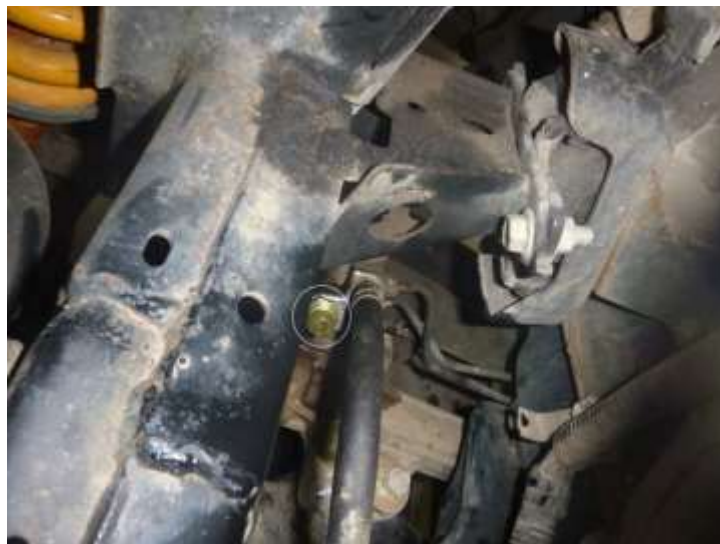
Image 4.1 Fit the gold plated MFC20401 adaptor fitting into the steering rack
