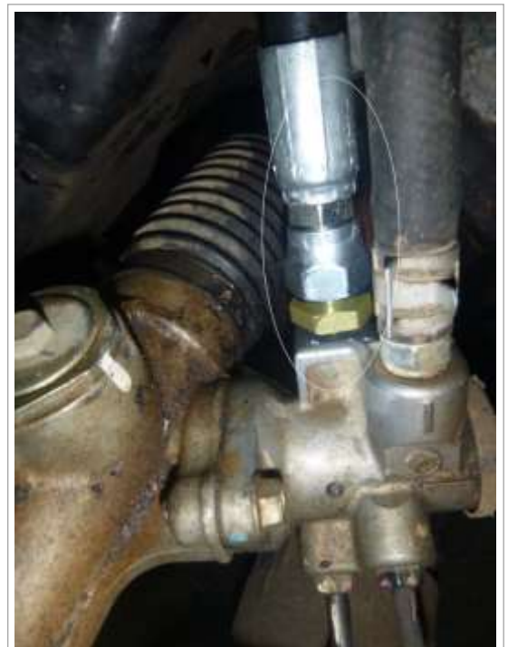
Image 4.2b Steering rack line fitted
