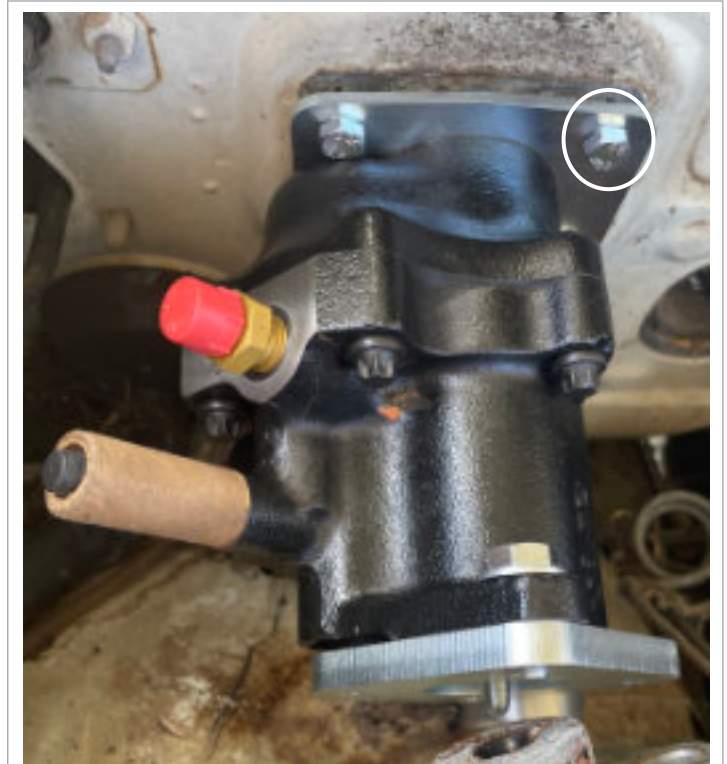
Image 3.2 Fit the two other bolts to hydro booster
