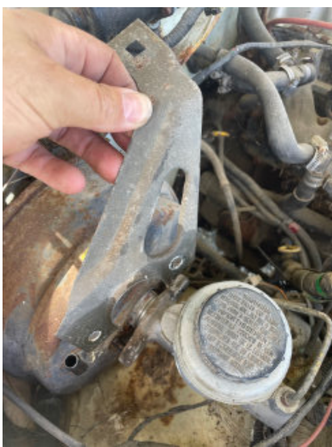
Image 1.2 Removal of 2 nuts, bracket & vacuum pipe.
