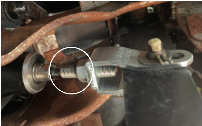
Image 3.5 Adjust the pedal saddle
