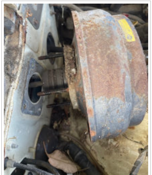
Image 1.3 Removal of 4 nuts & vacuum pipe.
