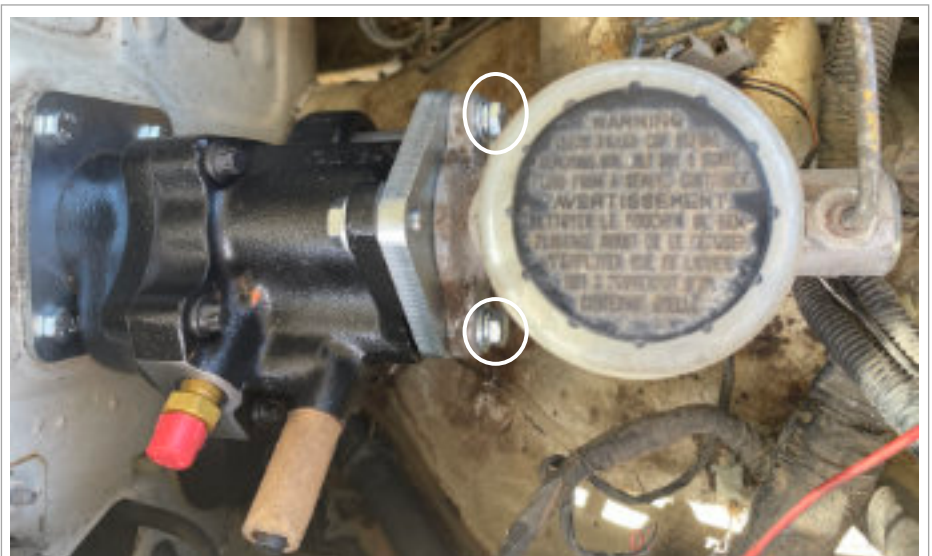
Image 3.6 Fit the master cylinder to the hydro booster
