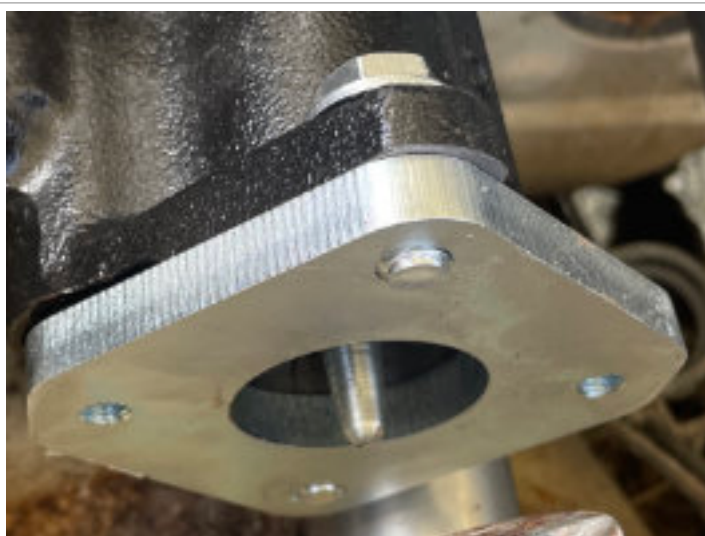
Image 2.1 Make sure the push rod is fitted in the hydro booster.
