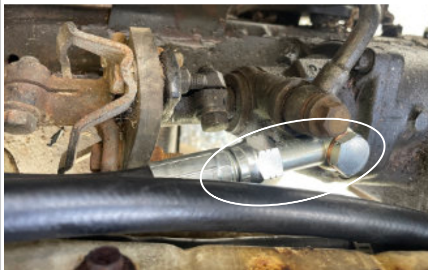
Image 4.2 Booster to power steering pump
