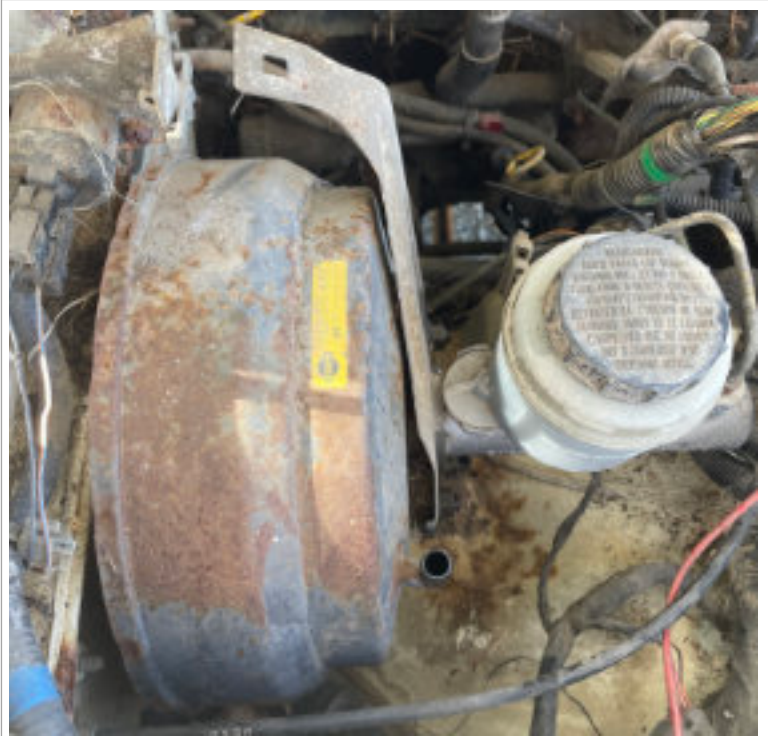
Image 1.1 Nissan factory brake booster and master cylinder setup.
