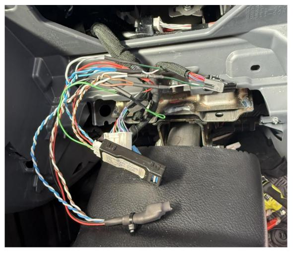
NOTE: Pictured is a shortened Speedo corrector loom. We recommend using the total length of wires supplied which will allow you to run the corrector out from behind the instrument cluster and adjust it during a test drive. The CAN interface module is designed to live behind the instrument cluster.
