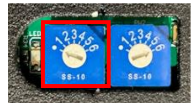
Figure 1 Left Rotary Switch for Measured Voltage Applications outlined in RED.
