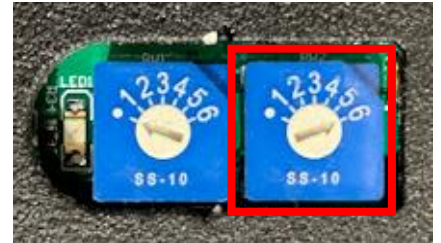
Right Rotary Switch for Off Delay Applications outlined in RED.
