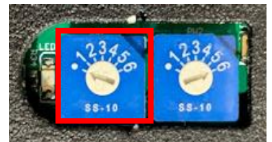
Left Rotary Switch for Measured Voltage Applications outlined in RED.
